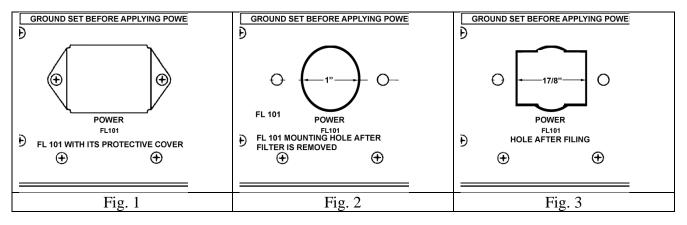
Fig. 1 shows the typical back of the receiver with the cover over FL 101. Fig 2 the hole with the filter removed and Fig. 3 the modified hole
